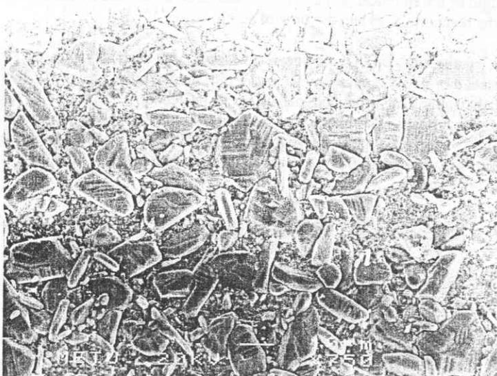
Figure 6. Typical SEM micrograph of sintered (1250°C, 17 h) BaTiO<sub>3</sub> samples with about 2 mol% excess of TiO<sub>2</sub> in the starting mixtures.
