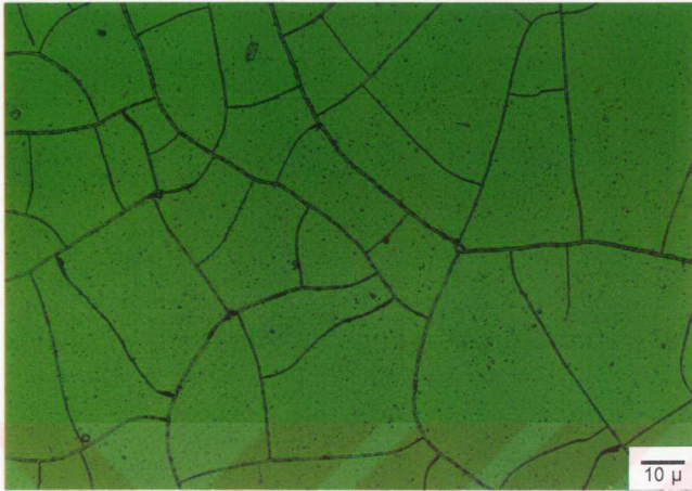
Fig. 4.7.a. Micrograph of the film produced from a mixture of HA and DW.
