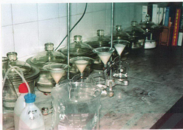
Fig. 3.1. Filtering of HA powders by gravitational draining, and desiccators with controlled relative humidity.
