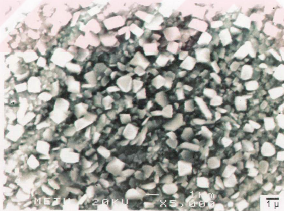
Fig. 4.9.d. SEM micrograph of 316L after heating at 840°C in an air atmosphere.
