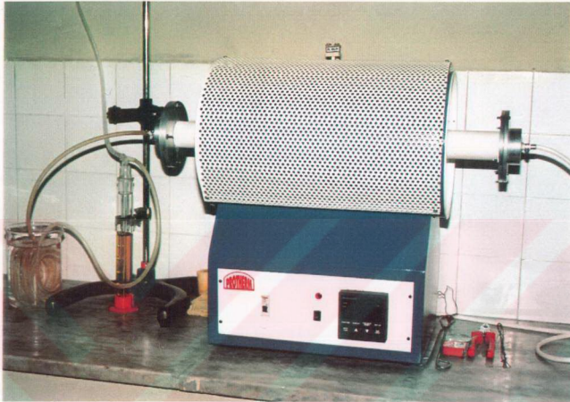
Fig. 3.5. Horizontal tube furnace used in the heat-treatment of coatings.
