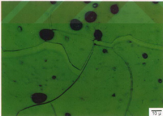
Fig. 4.7.b. Micrograph of the film produced from a mixture of GEL, HA & DW.
