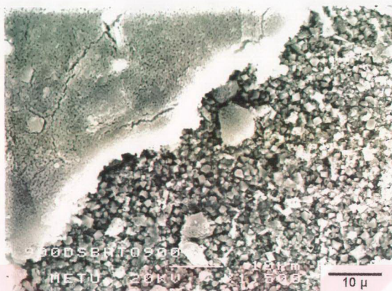
Fig. 4.4.a. SEM micrograph showing “unsuccessful” dip-coating trial on 316L.
