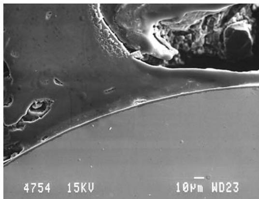
**Fig. 2** SEM micrograph of a cross section of MA956 alloy coated with  $\alpha$ -alumina implanted in the hind leg of a rat
