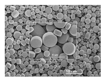
Materials with "biconvex micropill"-shaped particles are not yet reported in any other naturally-occurring or synthetic systems.
