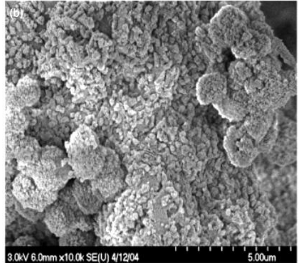
TTCP particles started their conversion to apatitic calcium phosphate only after 3 days of immersion in Tas-SBF at 37°C
