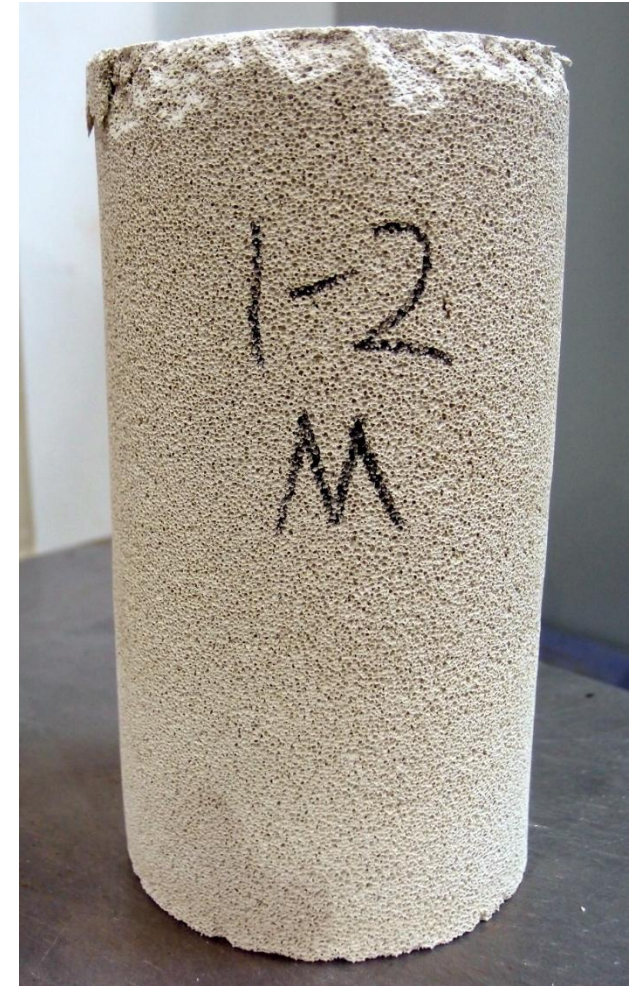
No catastrophic failure in the compressive strength-tested 20 cm tall, 10 cm diameter Solidia aerated sample
